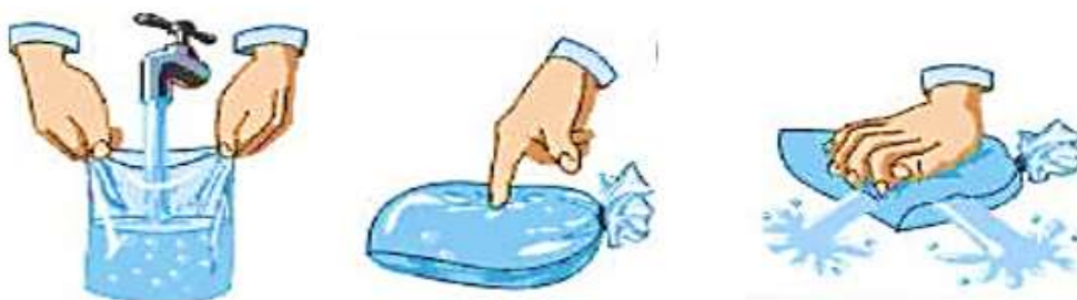
Figure 3. Experiment demonstrating hydrostatic pressure
