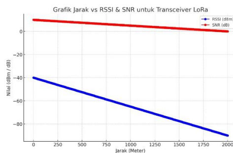
Figure 8. Distance, RSSI and SNR tests
